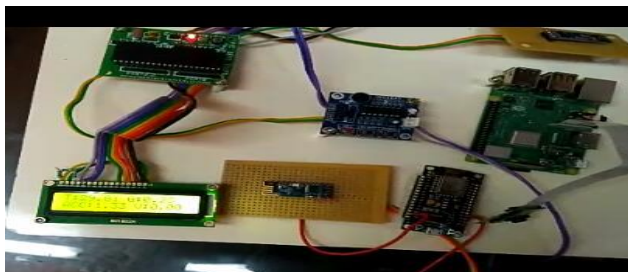
Fig-11: Hands on kit of Anti-Poaching System of Trees using WSN and IOT after detection
