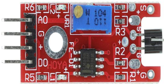
Fig.4. KY-036 Metal touch sensor
