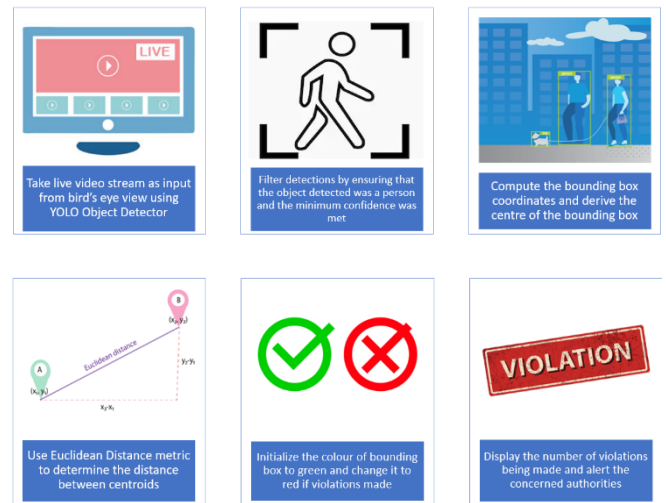
Fig-3: [Read from left-to-right] Working of Social Distancing Detector. This image displays the six significant steps that are necessary to understand the working of the model.
