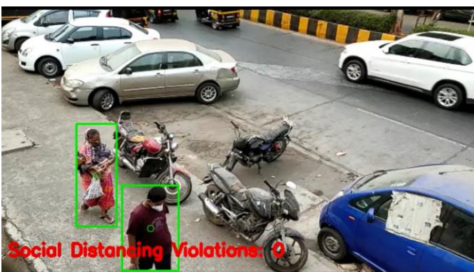
Fig-14: Snapshot of real time social distancing detection that shows zero number of violations being made by the pedestrians walking.
