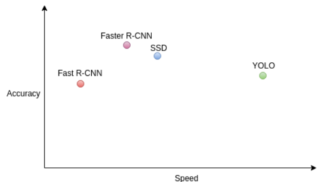
Fig-5: YOLO is faster than all the other object detection models which makes it suitable for real time object detection. (Image credit: Sayon Dutta)
