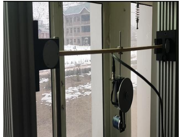
Fig-6: Experimental setup of pinned-pinned beam
