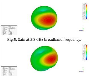
Fig.6. Gain at 5.5 GHz broadband frequency.
