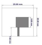
Fig.1a. Patch plane of proposed antenna.
