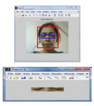
The system successfully detects the close eyes and alerts the driver to focus on driving by providing a beep.
