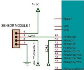
Fig -5: Connection of the module1 with Arduino
