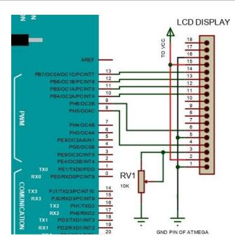
Fig -9: Connection of the LCD (16X2) with Arduino
