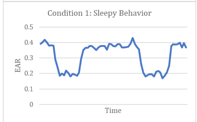
Chart-3 illustrates the EAR vs Time plot of the system which is tested under the daylight conditions as well, but where Infrared/Night vision is naturally off due to the abundance of light for the camera. The driver emulates normal blinks and has no facial accessories.
