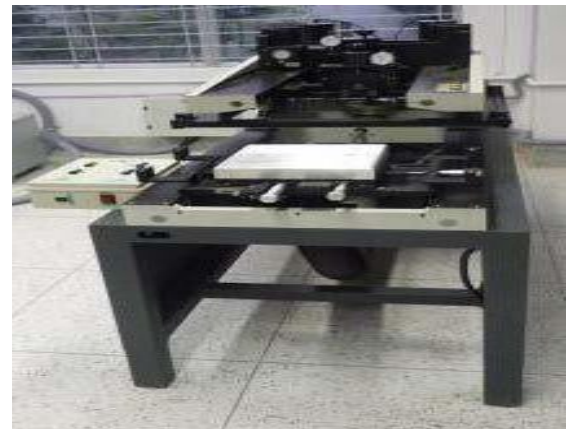
Figure 5: Screen printer for edge isolation
