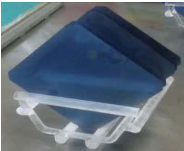
Figure 7: Phosphorous doped on P type Si wafer from diffusion chamber.
