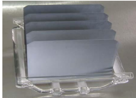
Figure 2: Starting p-type monocrystalline silicon wafer A. Cleaning and Texturing
