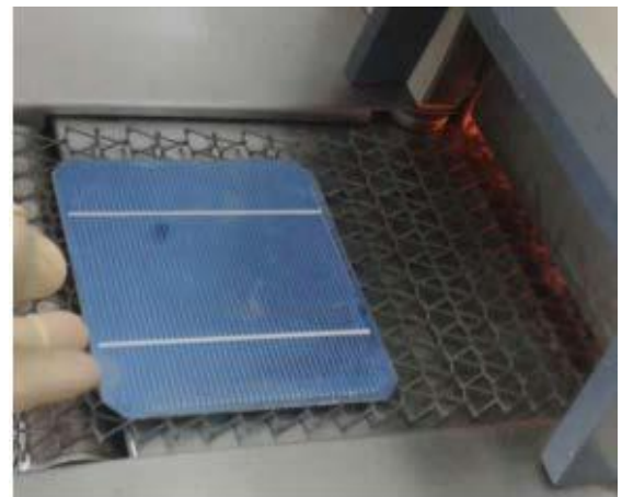
Figure 9: Contact firing at RTC furnace
