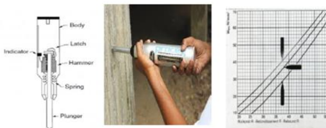
Fig -1: Rebound hammer testing and graph
