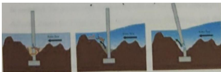
Debrts fill hole Light flood (erosion) Collapse
