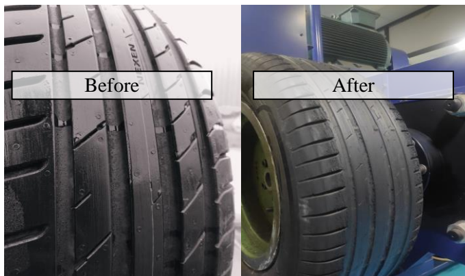
Figure-11 Photographs of same tyre before and after wear (after running for 40000 Km, Tyre Size: 205/65 R16 95W-A).
