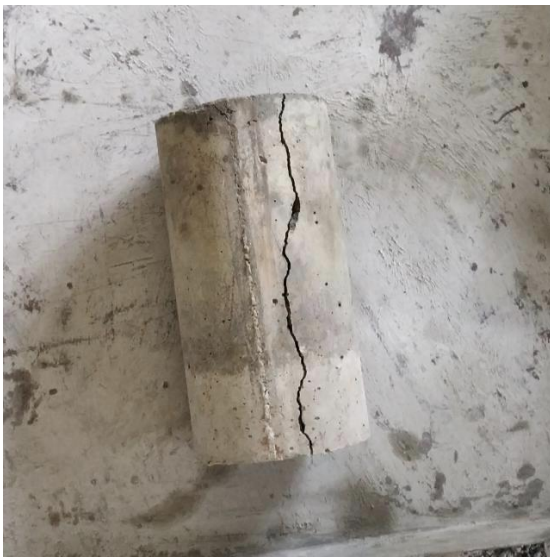
Fig-6: Cylinder after testing
