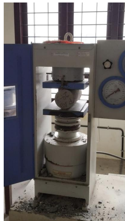
Fig-5: Cylinder kept for testing in CTM
