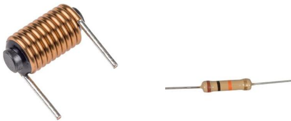
Figure 2: Inductor and 10k Resistor.
