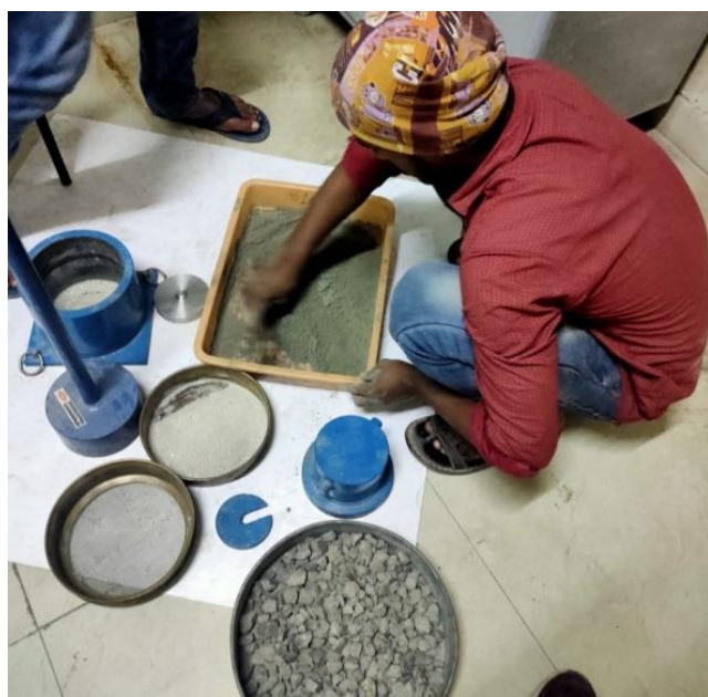
Figure 3.5, Mixing of Glass with Fine Aggregate
