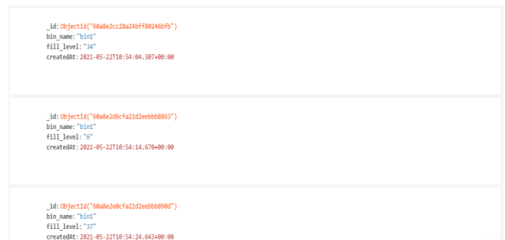
Fig -3: Fill level sensed by HC-SR04 pushed to MongoDB Atlas database
