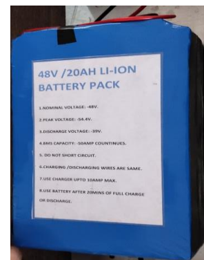
Figure -6: Battery Unit
