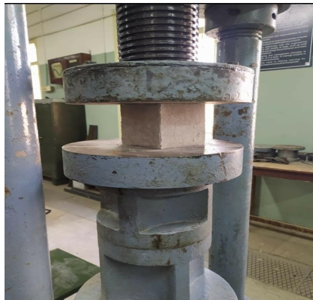
Fig-8: Compression testing of luminescent concrete cubes.
