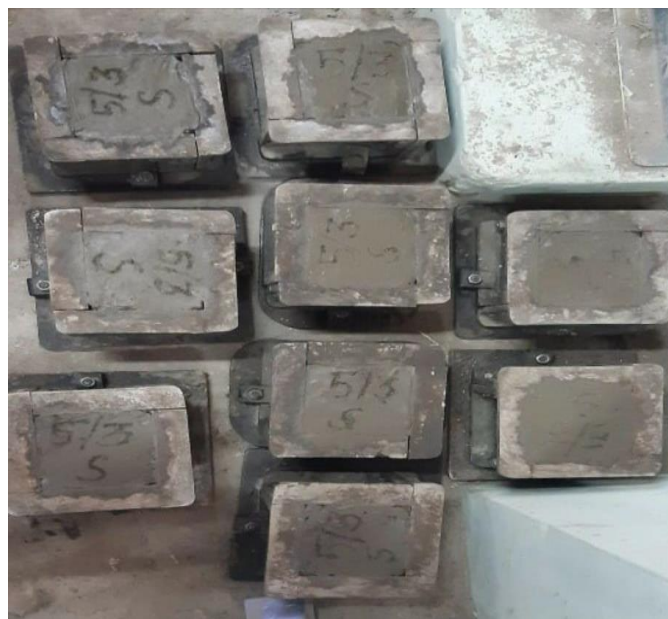
Fig-6: Setting of luminescent concrete.
