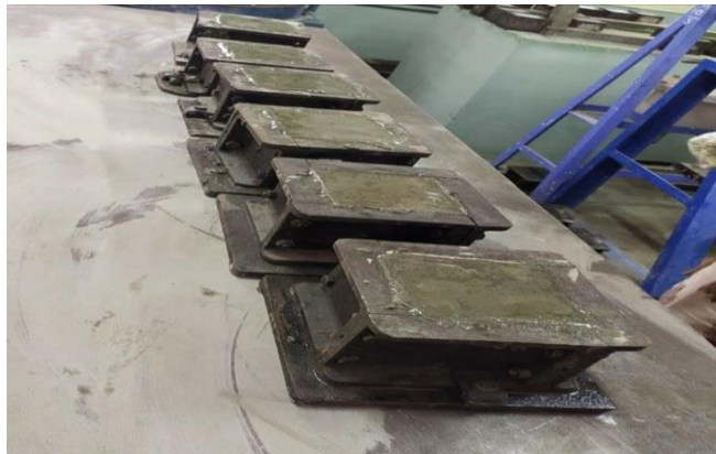
Fig -2: Casted cubes kept for vibration.
