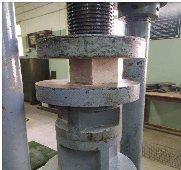
Fig-7: Compression testing of conventional concrete cubes.
