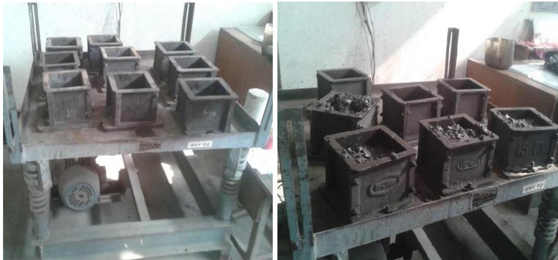
Fig. 3.1: Cube specimen on vibrating table
