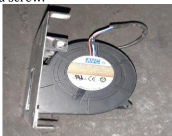
Fig-10: Centrifugal fan mounted on Aluminium Cover.
