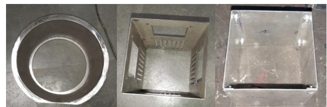
Fig-9: Hoop, Main Base, Aluminium Box after sheet metal cutting.
