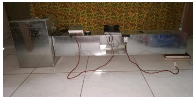
Fig-1: Setup of Water Extraction from Air
