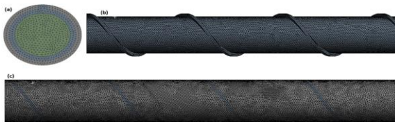
Fig -7: meshing of double pipe heat exchanger (a) Face side (b) Baffle (c) Volume Mesh
