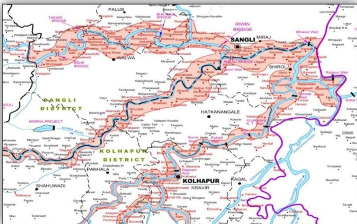
Fig.No.4.Flood spread area of Sangli District
