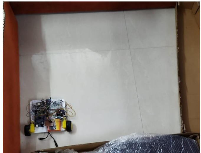
Fig -7.2: Robot while border following and mapping
