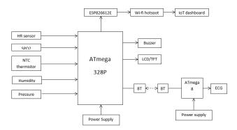
Our device consists of two parts, one is specifically for the ecg measurement and a main part which consist of the sensors and all the processing takes place in it. The ecg part is connected to the main part through bluetooth, It is done inorder to avoid the inconvenience (as there is possibility to accidentally disconnect the attachments as the patients move around) of the patients and also to measure the ecg more reliably.
