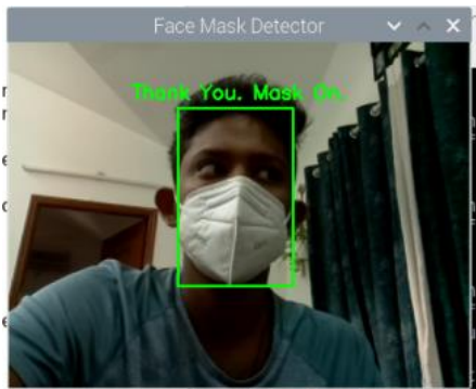
Figure 9. Face mask detected when the mask detection model is run on live stream with help of Raspberry Pi
