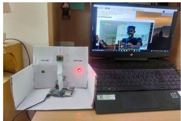
Figure 4. Red LED is turned ON when the human is detected on the right
