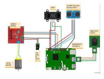
Raspberry Pi 4, Model B: Raspberry pi is the main computer used in the circuit. It uses a Broadcom BCM2711 SoC 1.5 GHz 64-bit quad-core processor. It has a standard 40-pin configuration which is used for various GPIO operations.
