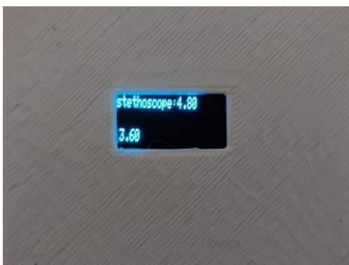
Fig. 11 The output voltage of MIC sensor and Battery is displayed correspondingly. The voltage of mic sensor changes according to the input analog value of audio signal. For the normal case of battery voltage, it keeps approximately 3.6 V. It decreases according to energy
