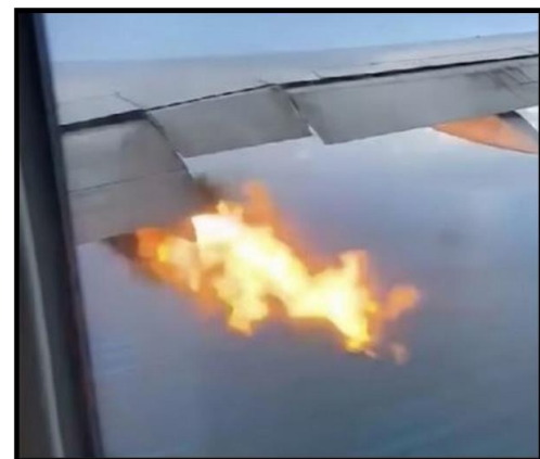
Fig 7 : Flame Out Observed from the Cabin Window on Boeing 777
