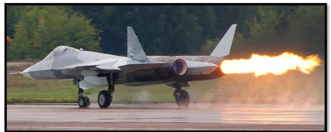
Fig 6 : Su-57 Suffering from a Compressor Stall
