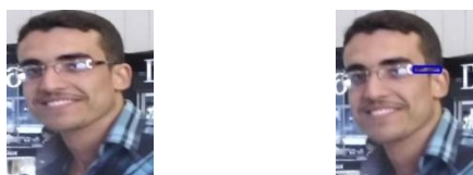
Figure-7: Viola-Jones showing False Positive in frontal image [Specs on Faces Dataset]
