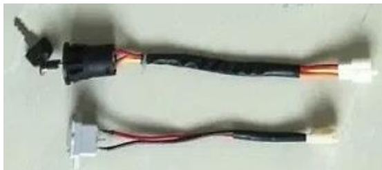
Fig-7: Ignition Switch
