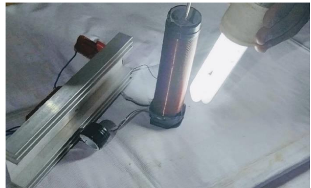
Fig.6.Tesla coil testing using Fluorescent Bulb
