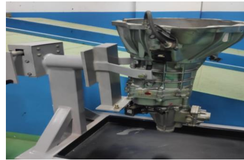
Fig-2: Load carrying element with Differential being the load.
