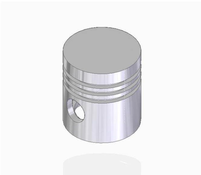
Fig 4: 3D model of Aluminium alloy cast 336
