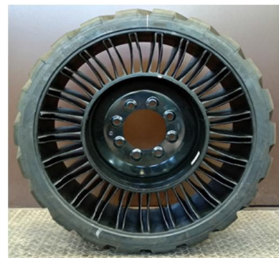
Fig -3: Michelin Tweel Tyre Design
