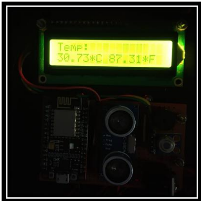
Fig -14: Temperature measurement in 16*2 LCD after displaying IP address
