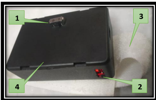
Fig -11: Hand gesture module placed over a Velcro strap
