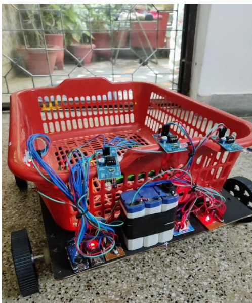
(ICs with photodiodes, wi-fi module, Arduino nano powered by 3 batteries)
