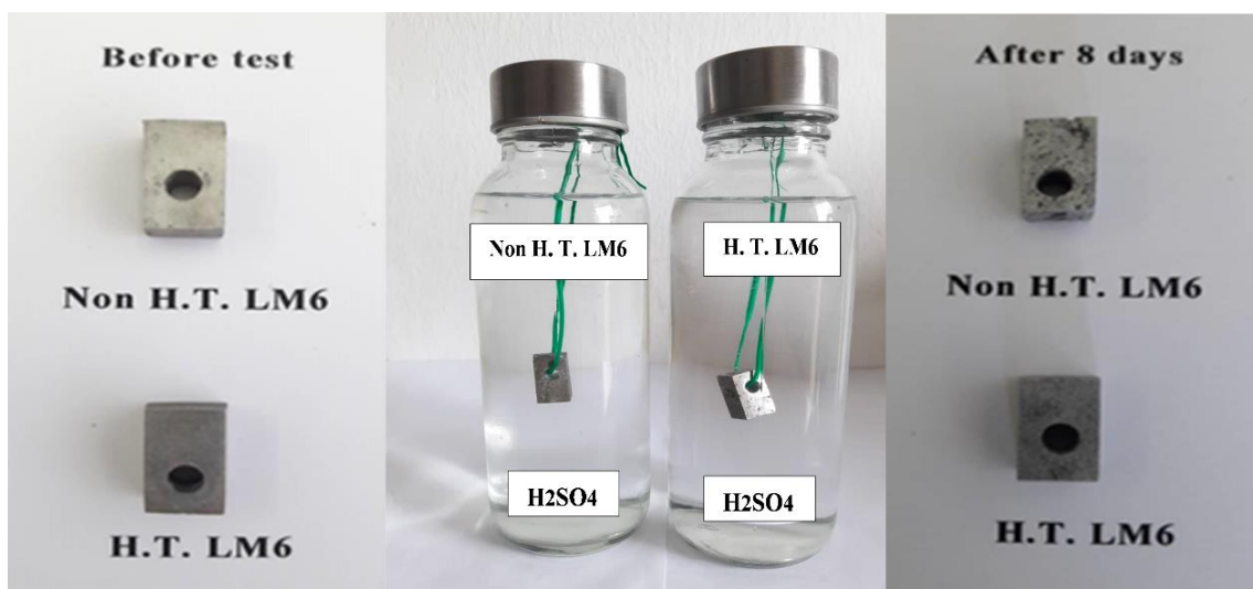
Fig- 2: Corrosion test steps immersion in acidic solution ( H_2SO_4 )
