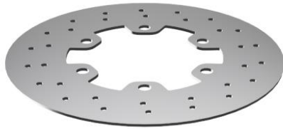
Fig -5: Rear brake disc design
