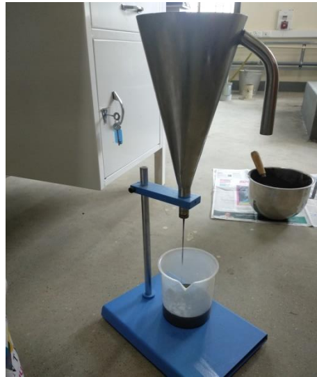
Fig. 3- Performing marsh cone test.
