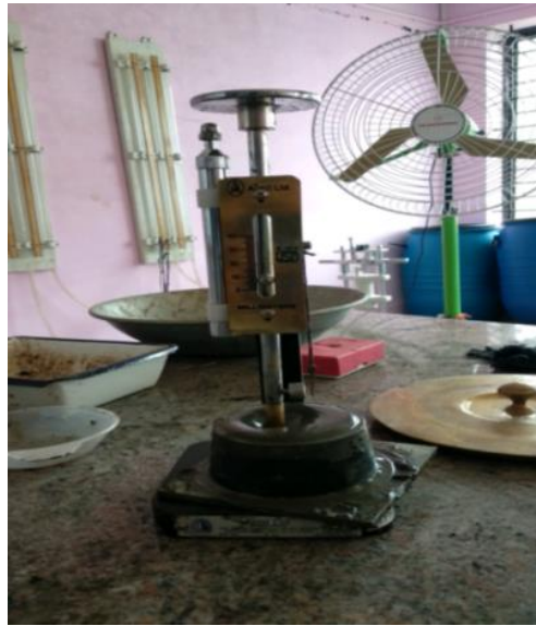
Fig. 1- Water demand test with SP using vicat's apparatus.
