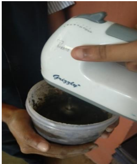
Fig. 2- Mixing of paste using cake mixer.
