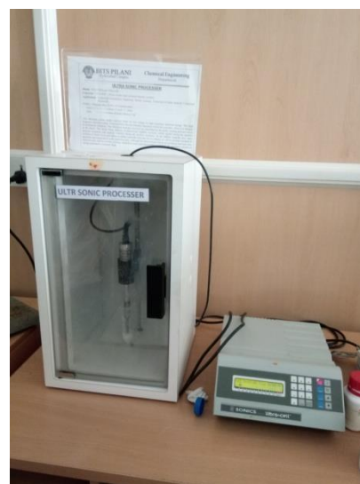
Fig 4.4: Probe Sonication for sample preparation
