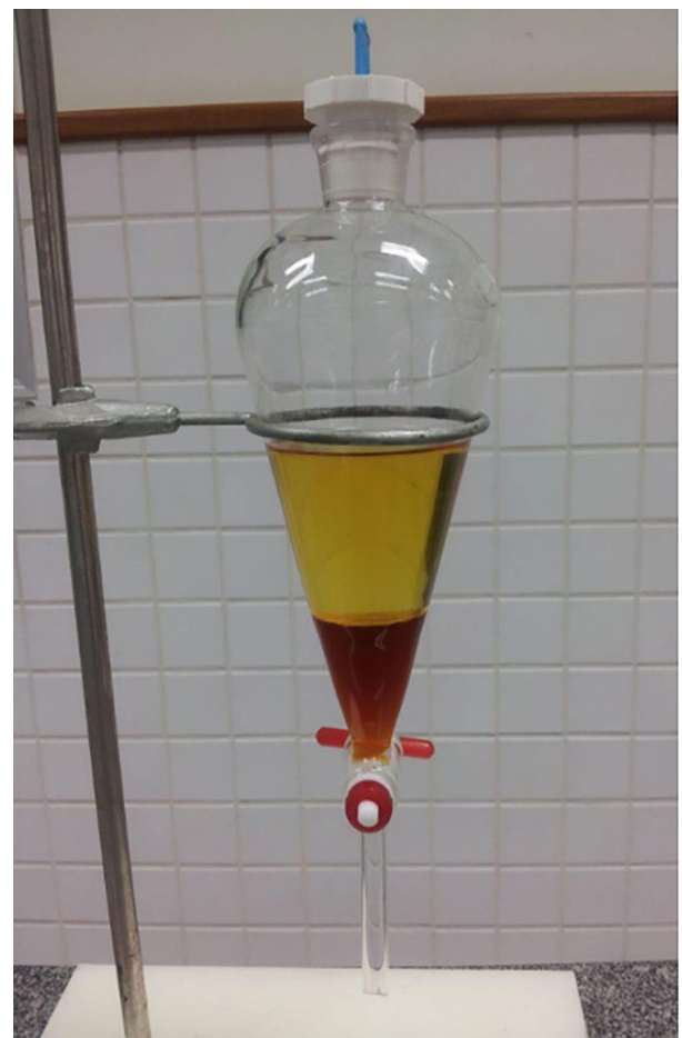
Fig 4.2: Separating funnel separating the sediments at the bottom
