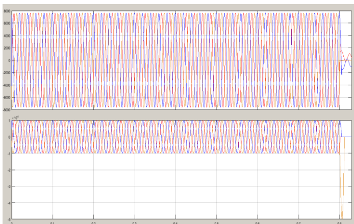
Fig-19: Three phase rms voltage and current of secondary side of transformer during LG-CG Line to ground fault at primary side at 0.8 second simulation time
