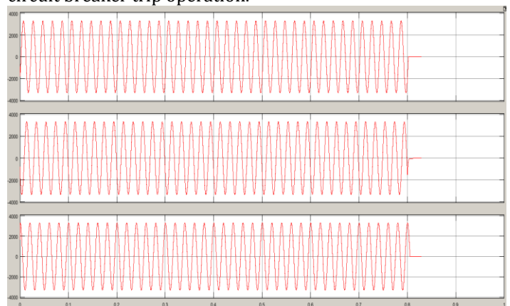
Fig-21: Three phase individual phases currents of secondary side of transformer during LG-BG line to ground fault at primary side at 0.8 second simulation time
