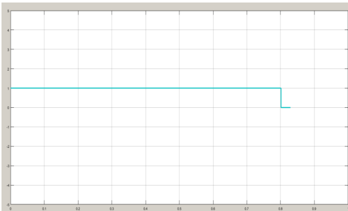
Fig-22: Trip signal generated during LLL-ACG Double line fault at primary side at 0.5 second simulation time for circuit breaker operation
