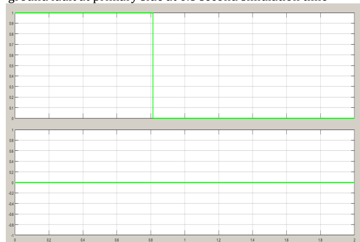
Fig-29: Trip signal generated during case-1 fault at 0.8 second simulation time
