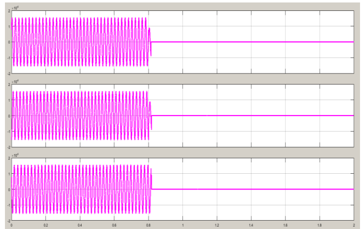
Fig-24: Three phase individual phases voltage of primary side of transformer during LG (AG) line to ground fault at primary side at 0.8 second simulation time
