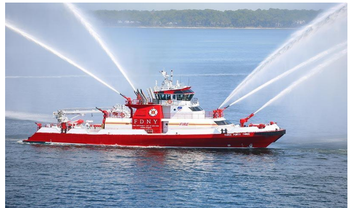
Figure 2 Application of water monitor
