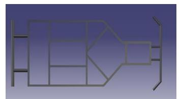
**Ansys software**. To investigate the field failure of 100Ton dumper theyintroduced gussets in failure area. After modification the chassis structurewas validated by linear static analysis andfound that the modified chassiswas safe.
