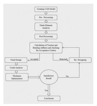
The method overview begins with creating a CAD model for the initial design of the chassis using design methodology rules.
