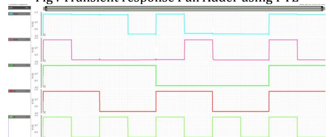
Fig : Transient response Full Adder using PTL
