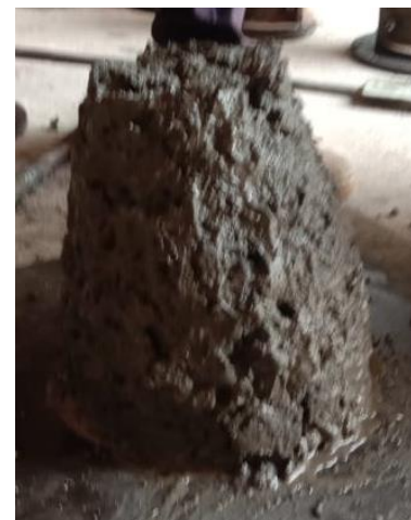
Fig. 2: Slump cone test.
