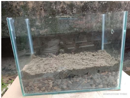
Fig -1: Construction of Wetland
