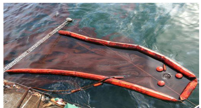
Fig-5: Cleaning of spilled oil using skimmers
