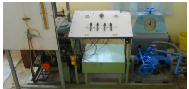
Estimation of Indicated Power, Brake Power and Friction Loses using Morse Test. [13]
