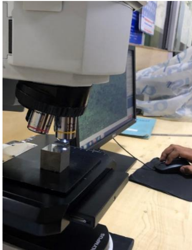
The microscope used for observing microstructure
