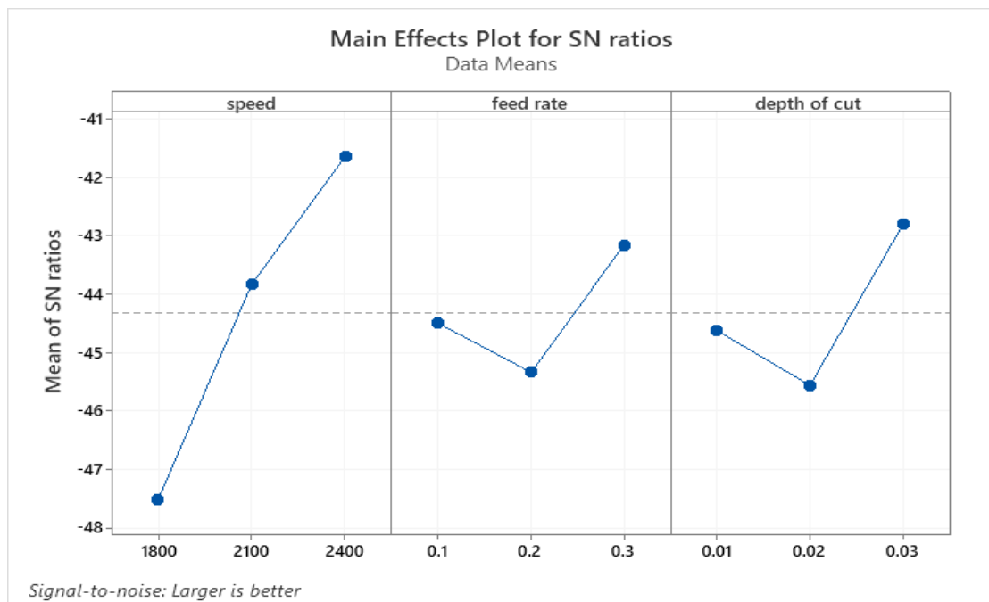
Fig. 14. Graph for S/N ratio obtained for CBN wheel (data from ref[2])
