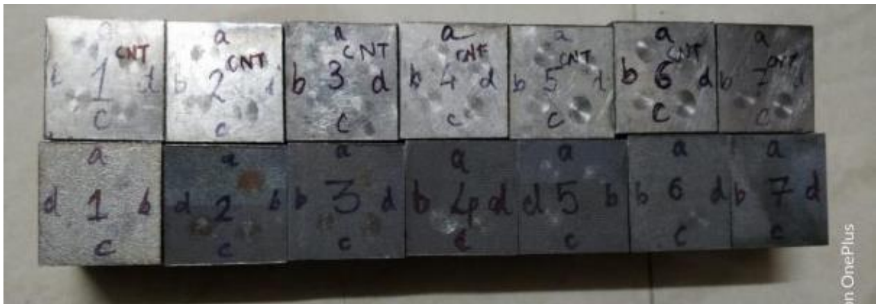
Titanium(Ti-6AL-4V) blocks marked and ready for the grinding process.
