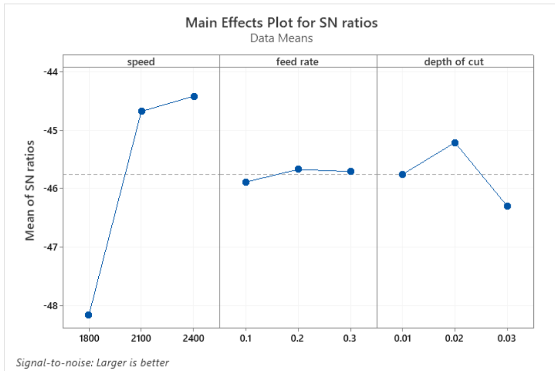
Main factor effect plot of MRR for 4% CNT- CBN wheel.(data from ref[2])
